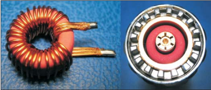
Figure 7 · Characterization of a 1/2-inch diameter core. Left: 10 turn winding presents sufficient impedance for a reliable measurement at LF. The trifilar winding minimizes winding loss. Right: The same core fitted in a coaxial short using a GR900 50 ohm connector, which provides a single turn for VHF measurement and will accept cores with an outside diameter of less than 14 mm.
